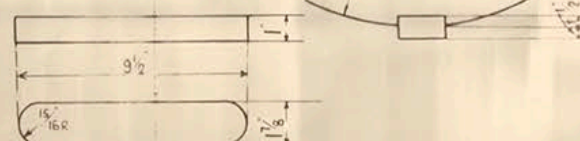
DETAIL OF KEY FOR VERT SHAFT SKEW WHEEL ON MAIN CRANKSHAFT
